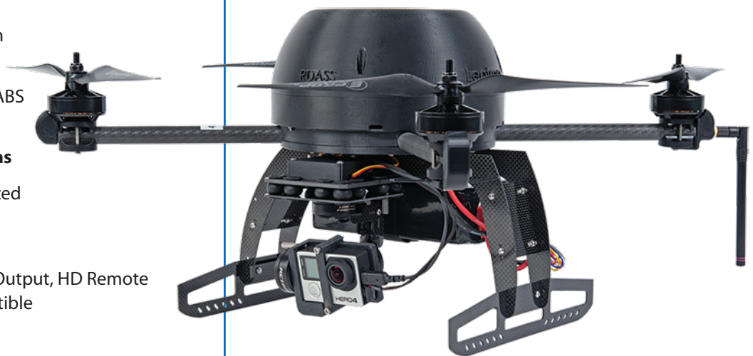
Leptron RDASS Precision with optional Stabilized Single-Camera setup using a GoPro Hero4 camera
